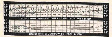
See how Moduflow smooths out the up-and-down temperatures caused by ordinary control systems. Shown above are actual temperature recordings taken in two identical houses — one with and one without Moduflow. Without Moduflow, temperature varies as much as 20 degrees from floor to ceiling
