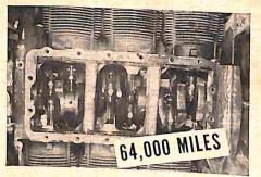
VEHICLE: 1964 Chevrolet CORVAN. OWNER: Jack Marchant, Clearwater, Florida. OIL: D-A Speed-Sport. RE-SULTS: Teardown showed engine to be very clean, no sludge anywhere, crankshaft and rod bearings had no measurable wear.
