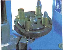
The RL 450 uses standard 7/8 x 14 dies. Rotary, sequential method of cartridge handling makes rapid consistent ammunition assembly a snap.
