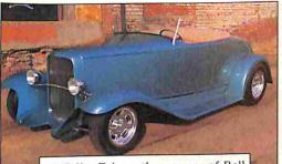
42 Jim Fairweather, owner of Bell Pech, always wanted a roadster, so he started with an Experi-Metal '32 Chevy body and fenders and built an extremely nice street rod with buggy spring suspension, '60s-style wheels and Corvette Sea Foam Green metallic paint.
