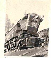
This 600-ton, coal-burning steamturbine-electric - world's largest single-unit locomotive—is Norfolk & Western's big gun in a cam-paign to put Old King Coal back on his railroad throne. For the story of the new challenge to Diesel supremacy, see page 150.
