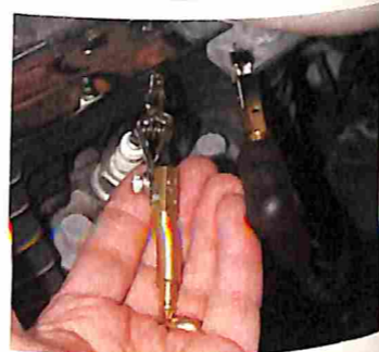
153 IGNITION GROUNDING PLUGS The safe way to handle ignition wires and spark plugs
