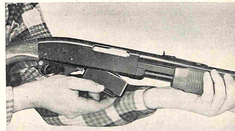
Box magazine on new Remington 760 holds four cartridges. To avoid trouble in loading, the following procedure is suggested: 1) insert round in chamber, 2) close action, and 3) insert full magazine
