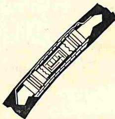
Precisely designed equalizing networks and amplifiers compensate for the loss in the cable every 40 miles and produce a communication highway 144 kc. wide.
