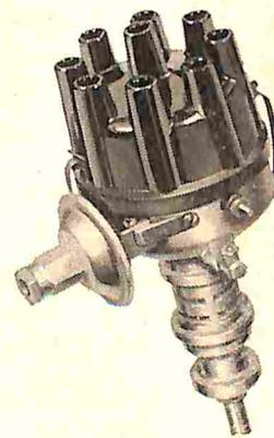
Centrifugal-vacuum distributor for V-8's has long-lived ventilated points. Breaker plate rotates on full ball bearings for split-second response to changing engine requirements.
